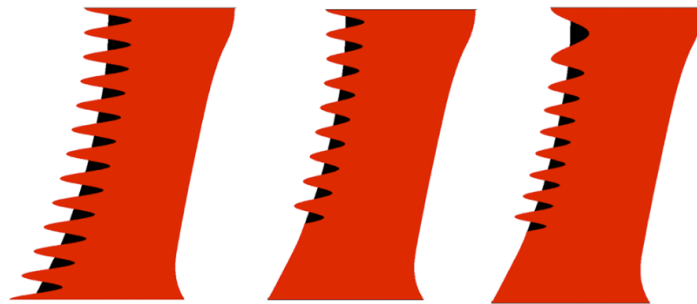
Figure VI.40: 2D low-noise OGV 2D designs: "GanzUniform" (left), "GanzUniformOpt" (middle) and "GanzRadialOpt" (right).
