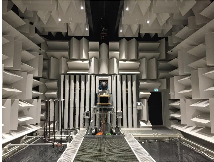
Figure II.12: Picture of the anechoic room at Centrale Lyon.
