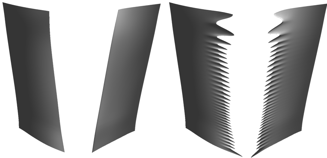
a) Suction side (ref.). b) Suction side (ref.). c) Suction side (serr.). d) Pressure side (serr.).
