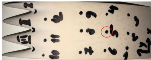
Figure VI.44: Locations of the roughness measurements (black dots).
