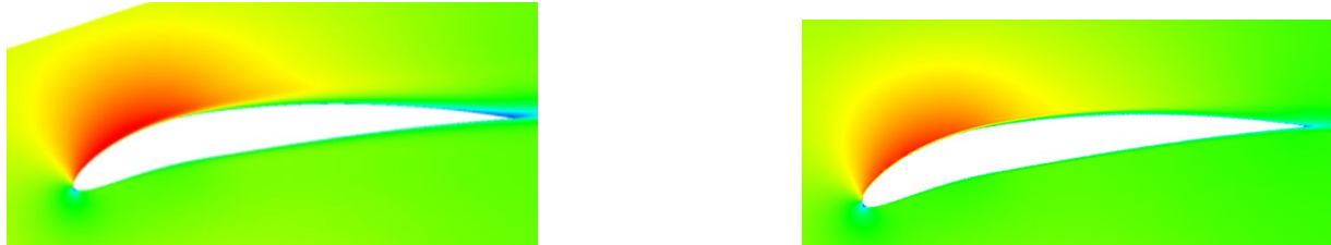
Figure V.44: Contour maps of mean Mach number for RANS (left) and LBM (right) computations. Levels between 0 and 0.5.
