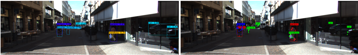
(a) YOLO network wrongly classifies reflections in the mirror as cars with high confidence (b) States of cars in the mirror are set as unknown (green) in our pipeline due to lack of consistently matched feature points for decision-making
