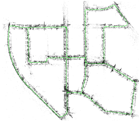
Figure 1.5 – The estimated vehicle trajectory and reconstructed sparse map of the scene with ORB-SLAM2 [12]
