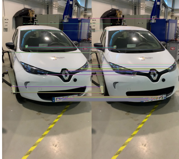
Figure 2.4 – The ORB features are detected and matched on two adjacent ZOE images
