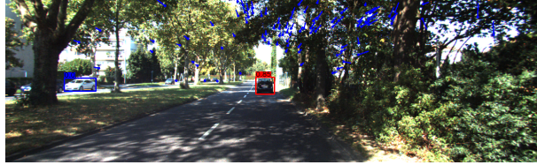
Figure 4.7 – The tiny moving object with degenerate motions (move along the epipolar plane) is successfully segmented with the FVB constraint
