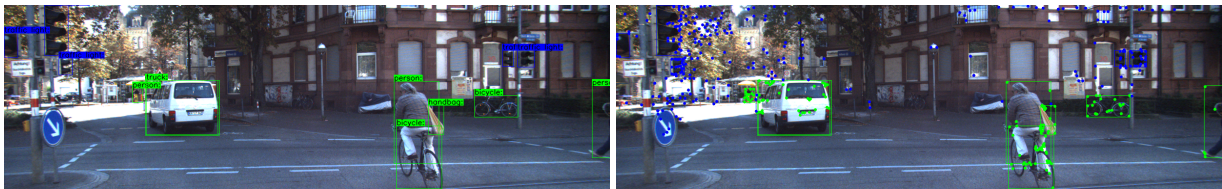
(a) Get the bounding boxes with semantic labels using yolo v4 detector
