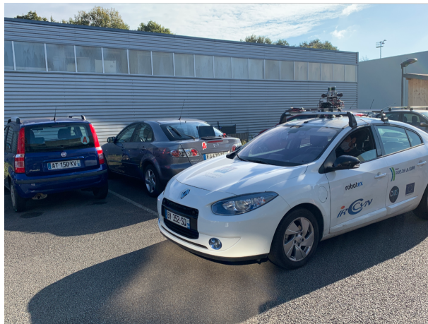
(b) The multi-sensor setup configured on the Renault vehicle in the LS2N dataset
