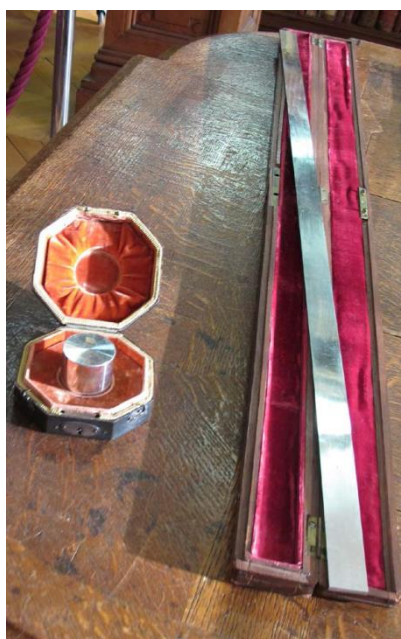
Fig. 13. Platinum standards kilogram and meter
