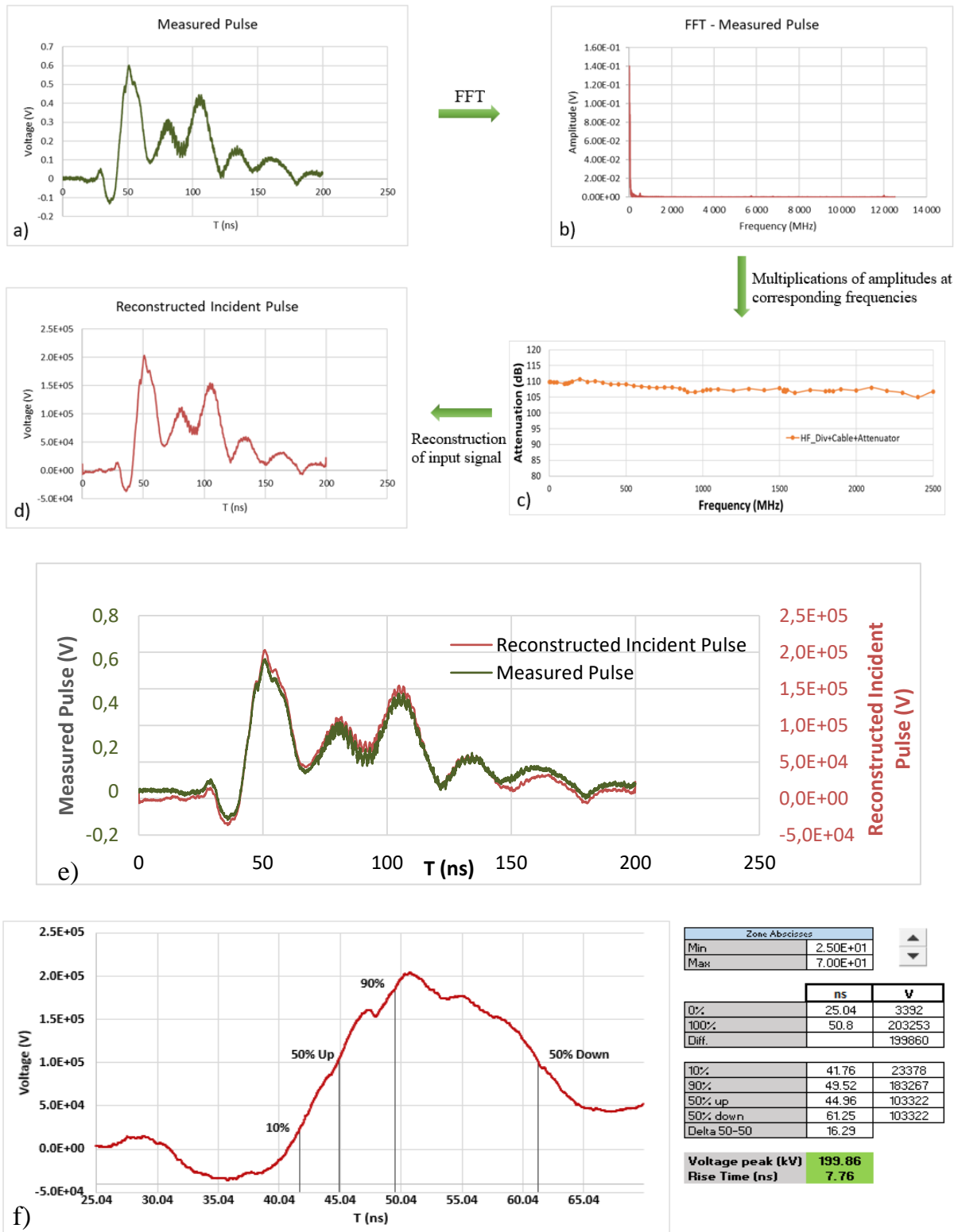
Fig. 59. A 200 kV output pulse of the Marx generator on a 50 Ω load, a) measured pulse at the output of the HPPNS measurement system; b) FFT of the measured pulse, which is multiplied to the corresponding attenuations in c); the reconstructed 200 kV input pulse generated by the Marx generator is presented in d); e) superposition of the measured and reconstructed pulses and f) rise time and voltage peak measurements of the reconstructed incident pulse
