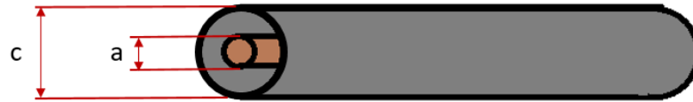
Fig. 18. Section of coaxial transmission line showing the diameter of the inner conductor a and the shielding diameter c
