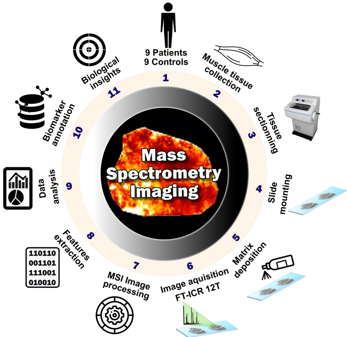
Supplementary Figure 11. General overview of mass spectrometry imaging workflow. (1) Patient selection; (2) Tissue sampling; (3) Tissue sectioning using a cryomicrotome; (4) Tissue section fixed to the sample probe; (5) Homogenous deposition of matrices using an automatic sprayer; (6) MSI data acquisition using an FT-ICR 12T Solarix Bruker; (7) Mass spectrometry imaging datasets (raw data files) were processed; (8) Raw data were converted into data matrices, including ion mass-to-charge ratios ( m/z ), spatial localization and relative intensity for each ion image, were generated using SCiLs Lab software; (9) Data analysis workflow for comparative analysis to extract the differential metabolic patterns; (10) Annotation of the discriminant features by interrogation mass spectrometry databases; (11) Interpretation of the data according to clinical and biological contexts.
