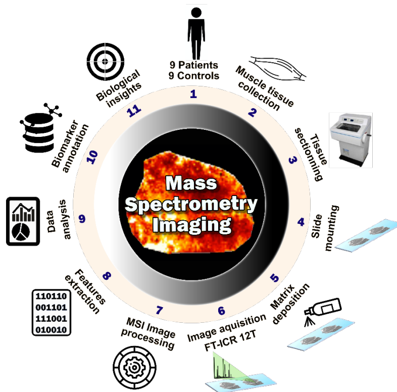
Figure 9 : General overview of mass spectrometry imaging workflow. (1) Patient selection; (2) Tissue sampling; (3) Tissue sectioning using a cryomicrotome; (4) Tissue section fixed to the sample probe; (5) Homogenous deposition of matrices using an automatic sprayer; (6) MSI data acquisition using an FT-ICR 12T Solarix Bruker; (7) Mass spectrometry imaging datasets (raw data files) were processed; (8) Raw data were converted into data matrices, including ion mass-to-charge ratios ( m/z ), spatial localization and relative intensity for each ion image, were generated using SCiLs Lab software; (9) Data analysis workflow for comparative analysis to extract the differential metabolic patterns; (10) Annotation of the discriminant features by interrogation mass spectrometry databases; (11) Interpretation of the data according to clinical and biological contexts.
