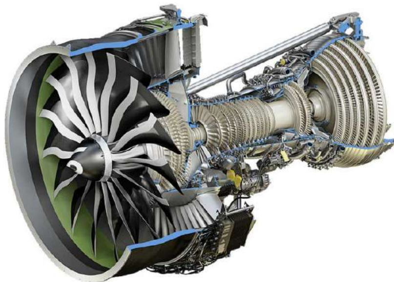
Figure 1.1: Representation of a modern gas turbine engine: Cross-sectional view of GE9X
