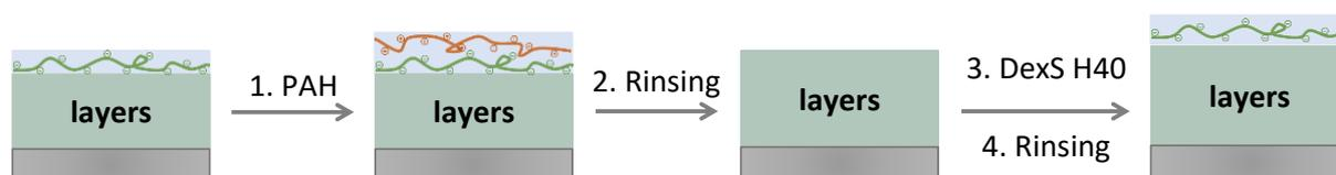
**Figure 3.19.** Proposed mechanism for the build-up of (PAH/DexS H40) PEMs starting from bilayer 4 on PEMs previously ending with DexS.
