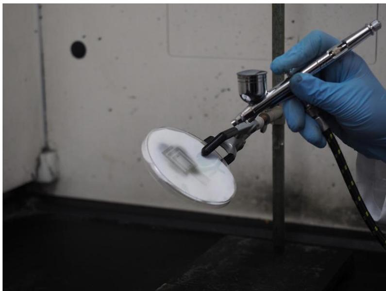
Figure 1.3: A spray-on nanoantenna. Source: Sarycheva et al. (2018).
