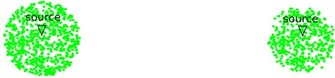
Figure 4.2: The communication range of the source hop without (left) and with the shadowing (right).
