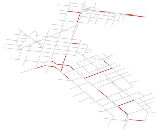
FIG. 2.8 – Selected links location in Athens network (grey links: all links in the network, red links: selected links for assessment)
