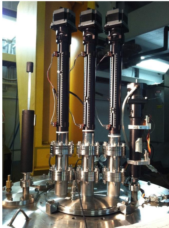
Figure 14. Three telescoping arms attached to the ladders allowing the remote control over them. Reprinted from ref. [113].
