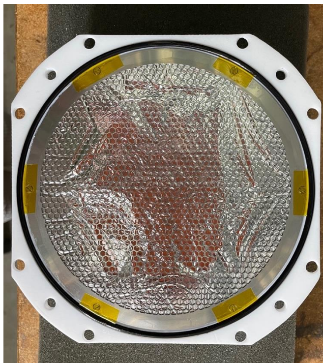
Figure 19. Aluminized Mylar window dismounted from the sRTC.
