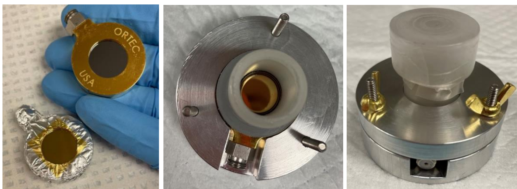
Figure 20. Silicon and gold-coated silicon detectors (left image), “chimney” placed onto the gold-coated silicon detector (center image), and the sealed “chimney” (right image).
