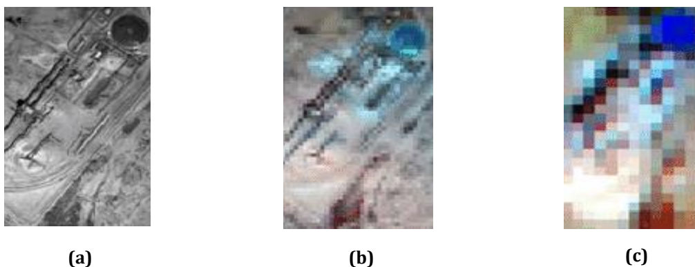
Figure 24 A comparison of spatial resolution between (a) panchromatic (b) multispectral (c) hyperspectral imagery ( Borstad et al., 2004 ).
