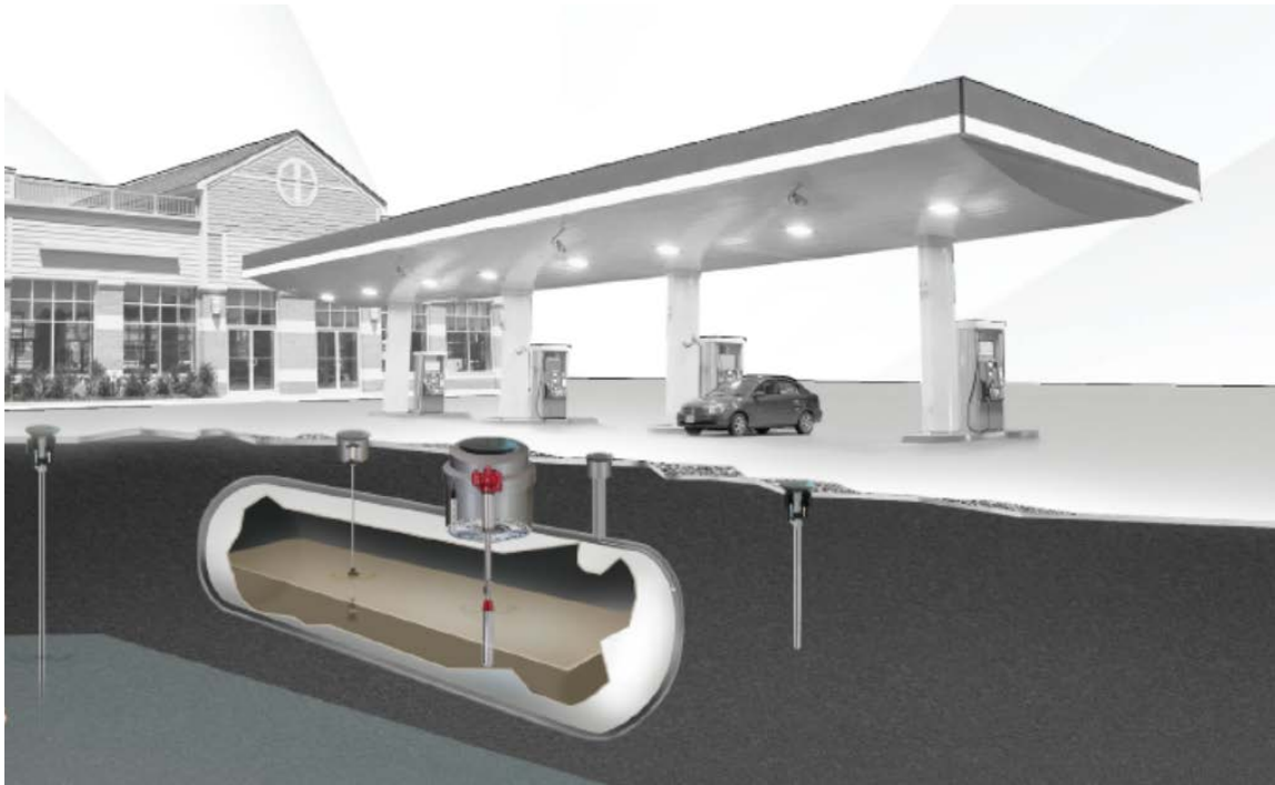
Figure 23: Illustration of an underground storage tank and possible monitoring and testing equipment for volumetric tightness tests (such as gages in the tank) or for other, external types of assessment (vapor monitoring well, groundwater well) from Veeder-root, a global supplier of tank gaging systems 13 .
