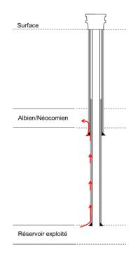
Figure 24: Microannulus leakage scenario considered in Vernoux and Manceau (2017)
