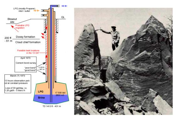
Figure 11 : Elk city blow out. Schematic of the leakage scenario (in red) and summary of the postincident investigations (left, from Réveillère et al., 2018) and of the results of the LPG blow out – without ignitio - at the surface (right, from Fay, 1973)
