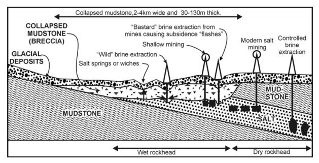
Figure 6: Cross-section through a typical Cheshire Triassic salt area showing past and present brine production techniques. From Cooper (2002)
