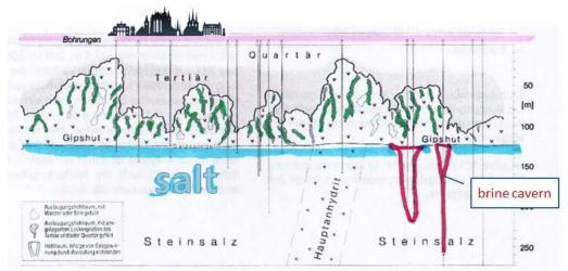
Figure 2: Section of a salt dome with 2 caverns without salt roof (in red contour) due to uncontrolled wild brining. From Crotogino and Wilke (2014)
