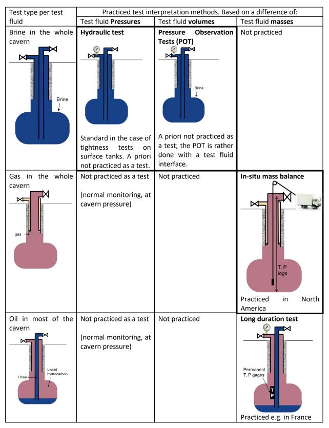
Table 5: main types of salt cavern tightness tests, or MITs, when the test fluid occupies a small volume relatively to the cavern volume, per type of test fluid and per interpretation method. Formulations of the Calculated Leak Rate (CLR) and of the Minimum Detectable Leak Rate (MDLR) are exposed in Section 4 for bold boxes cases.
