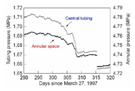
Figure 17. Annular Space and Tubing Pressure During a Well Leak. The two curves are parallel before Day 293 (no leak) and after Day 315 (leak repaired). Not in between, due to a surface leak at the wellhead. From Van Sambeek et al. (2005)
