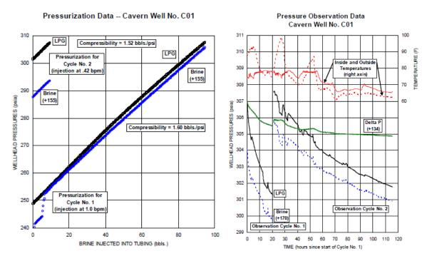
Figure 15. Left: the cavern compressibility is measured during the pressurisation<sup>10</sup> Right: Pressure decay during the test<sup>11</sup>. From Theil and Russel, 2004.
