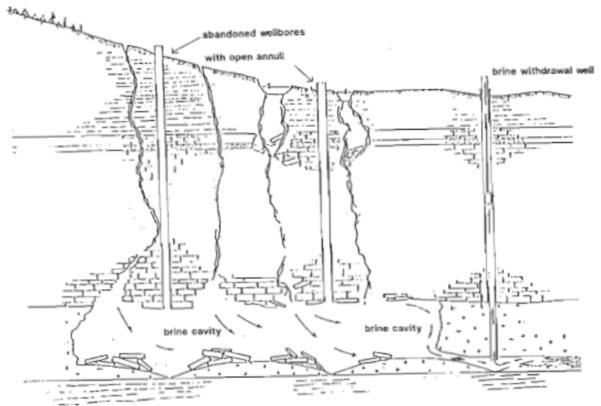
Figure 8 : schematic illustration of the Wild brining mining method applied at Tully valley. Brine cavity is recharged by groundwater through a flow in intentionaly open wellbores (after the casings have been pulled out), as well as fracture associated with subsidence. Brine is probably produced using air lift. From Stanford (1996).
