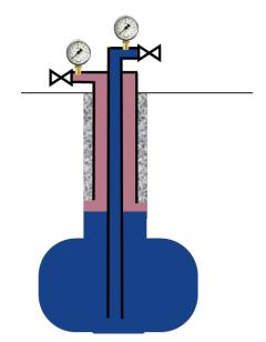
Figure 34. Cavern and monitoring used during a Pressure Difference Observation Test (PDO)
