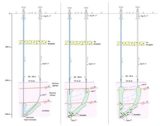
Figure 10: Schematic cross section of subsequent phases of salt leaching in Vauvert, France, by means of a doublet. Water injected in the well on the left circulated through cracks in the salt, dissolving it, and is produced by the well on the right. From Duquesnoy et al., 2013.
