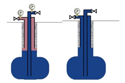
Figure 15. Cavern and main monitoring equipement during a POT. In the most referenced cases, POT is done with an oil-brine interface lowered down to below the casing shoe. But it could also be done with a cavern fully filled with brine, or with nitrogen instead of oil.
