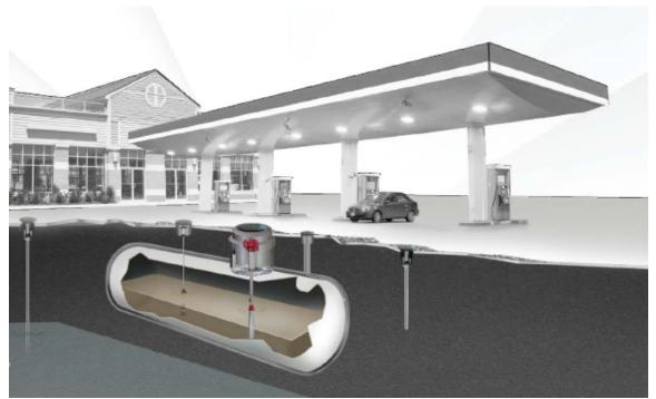
Figure 23: Illustration of an underground storage tank and possible monitoring and testing equipment for volumetric tightness tests (such as gages in the tank) or for other, external types of assessment (vapor monitoring well, groundwater well) from Veeder-root, a global supplier of tank gaging systems<sup>13</sup>.
