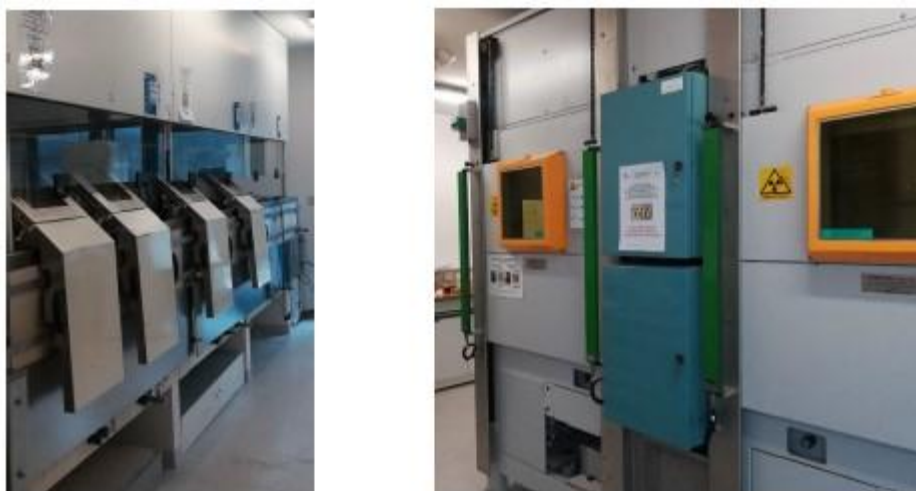
Figure 42 : Fume hood equipped with 5 cm lead-shielded (left) and hot cell (right).
