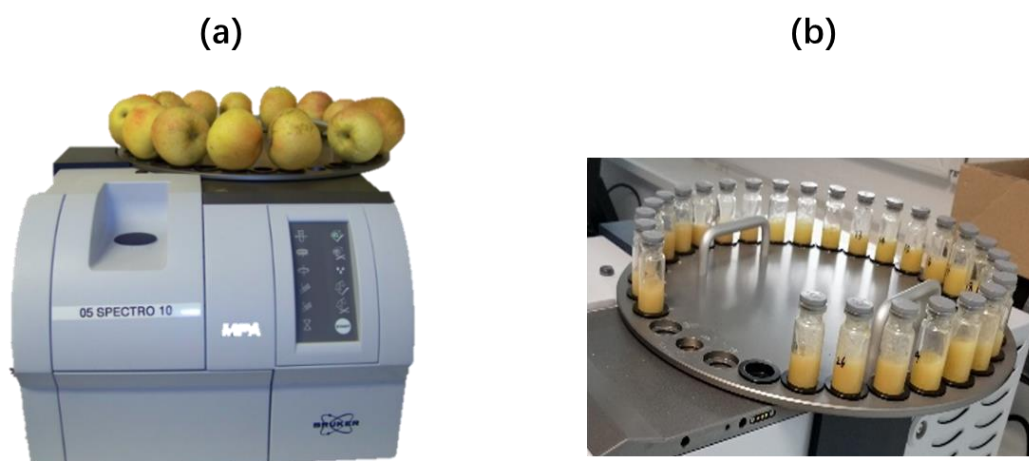
Fig. 14. An example of the measurements on (a) apple and (b) purees using the NIR spectrometer.
