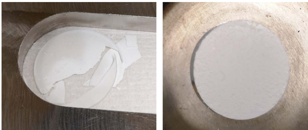
Fig. 3.8 Photos of a damaged pellet (left) and a complete pellet (right) during the recovery process.
