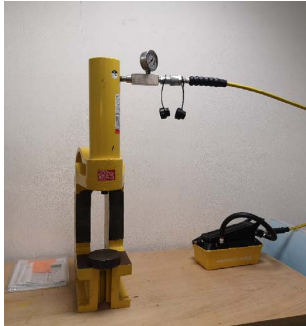
Fig. 3.1 Hydraulic press used in this work, the maximum capacity is 950 Mpa for a 20-mm-diameter-pellet.
