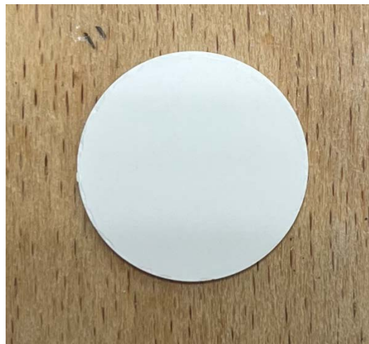
Fig. 3.18 Photo of the pellet made of enriched ^{155}Gd_2O_3 .
