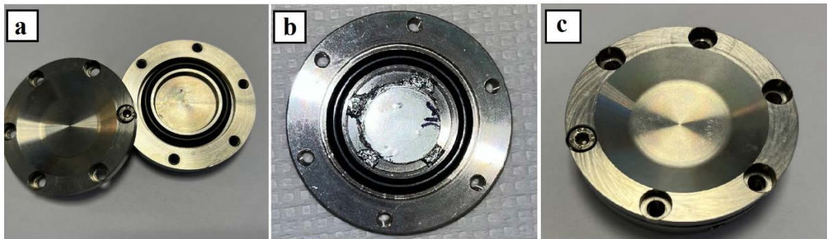
Fig. 4.31 The capsule and the assembly of the target. a: empty capsule; b: assembly of enriched targets fixed by Al balls and natural target; c: closed capsule.
