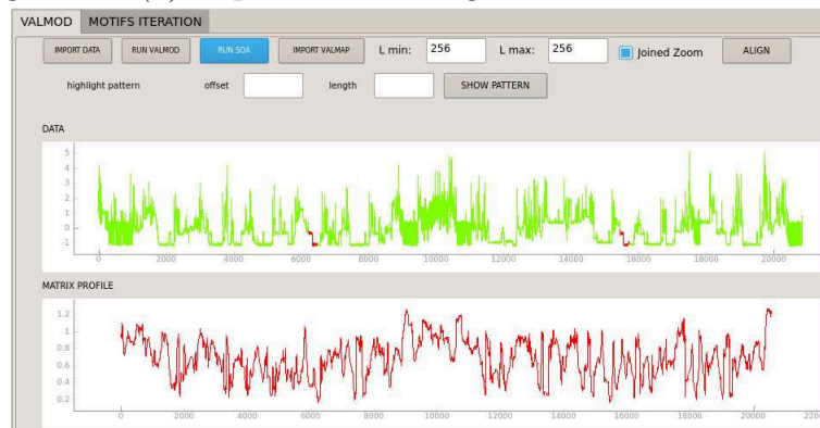
Figure 6.6: GUI interface of the prototype, Top - k motifs iteration. (a) Top-1 motif of length 256. (b) Top-1 motif of length 490.
