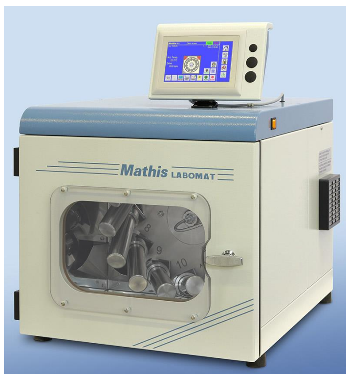
Figure 3. 7 Mathis LABOMAT dyeing machine (laboratory scale)
