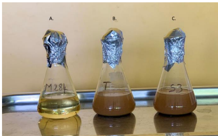
Fig. 1. Photos of the Erlenmeyer flasks used in the study of Mn-solubilisation. A. Erlenmeyer flasks containing only 284 culture medium, B. Erlenmeyer flasks containing 284 culture medium and sterilised red gypsum, C. Erlenmeyer flasks containing 284 culture medium, sterilised red gypsum, and bacterial culture.
