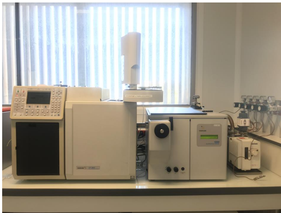
Fig. A.7 Varian CP-3800 gas chromatograph/ Varian 1200 quadrupole Mass Spectrometer Gas chromatography/mass spectrometry (GC/MS) analysis
