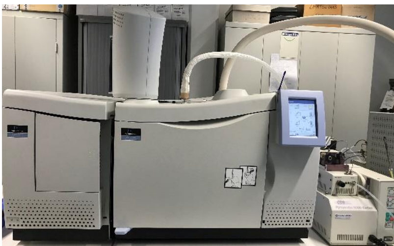
Fig. A.3 Perkin Elmer Clarus 680 Gas Chromatograph/ Perkin Elmer Clarus Mass Spectrometry for pyrolysis-gas chromatography/mass spectrometry (Py-GC/MS)
