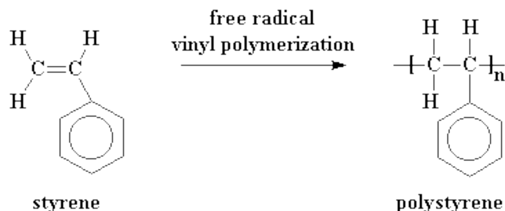
Fig. 1.7 Polymerization of styrene monomer to form polystyrene
