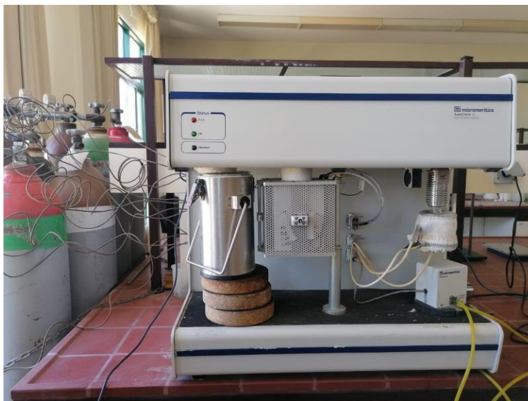
Fig. A.5 Micromeritics Autochem II chemisorption analyzer for H 2 -TPR and CO 2 -TPD analyses
