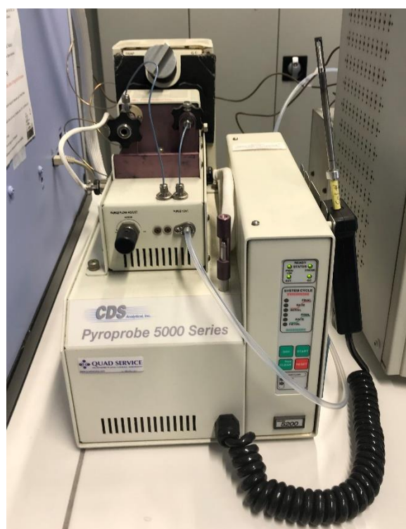
Fig. A.2: Plastic pyrolyzer CDS pyroprobe 5000 series linked to the injection port of the gas chromatograph
