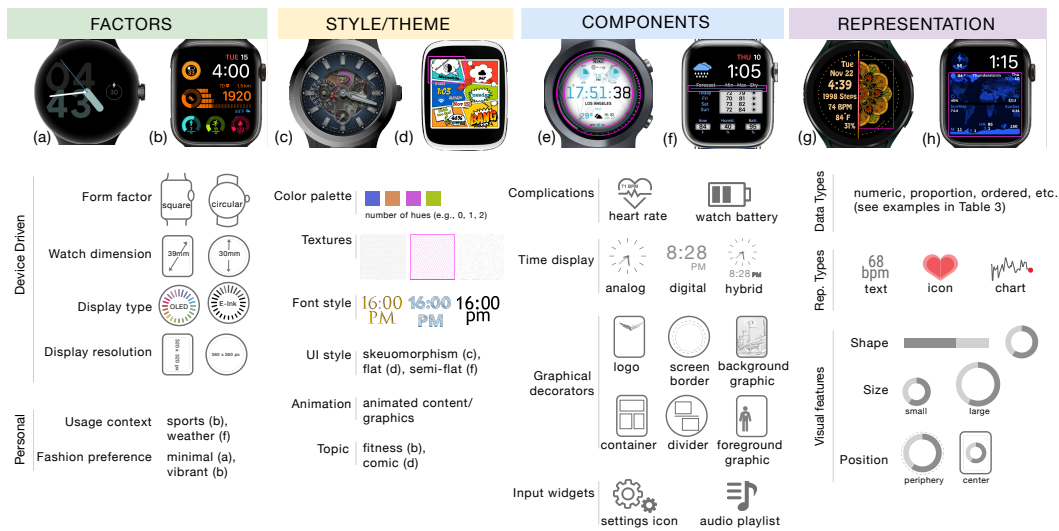
Fig. 5.1: The dimensions of our smartwatch face design space with examples. Watch face images (a, b, and f) indicate personal fashion preference as a factor; watch face images (c, d, and f) show examples of watch face design styles; and other watch faces (c to h) regions highlighted in magenta color are – a logo (c), a container (d), a screen border (e), a divider (f), a foreground graphic (g), and a background graphic (h). Figure acknowledgements can be found in Section 8.1.
