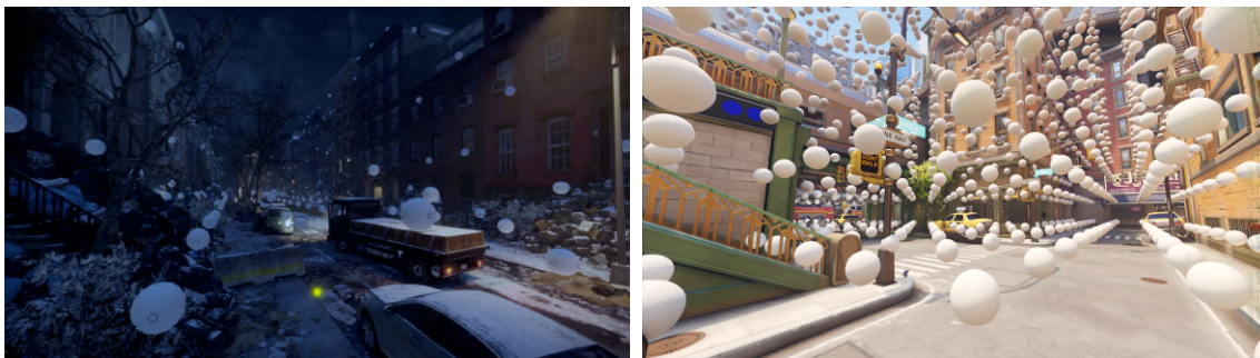
Figure 1.7: For dynamic object, global illumination in Tom Clancy's The Division [Mas16] (left) and Overwatch 2 [Bli22] (right) is captured by a set of probes, represented by white spheres, and the illumination is interpolated between a subset of probes closes to the shading point.
