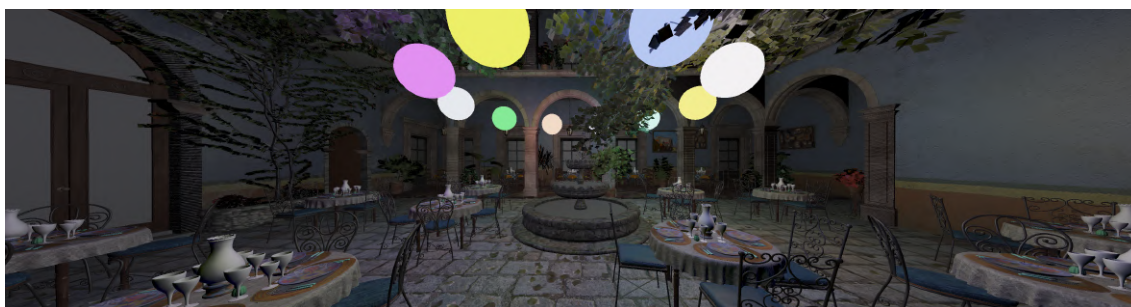
Figure 3.1: San-miguel with only 10 spherical lights whose projection is computed on 10 SH bands. Image rendered in 69ms with the resolution 3400×900.
