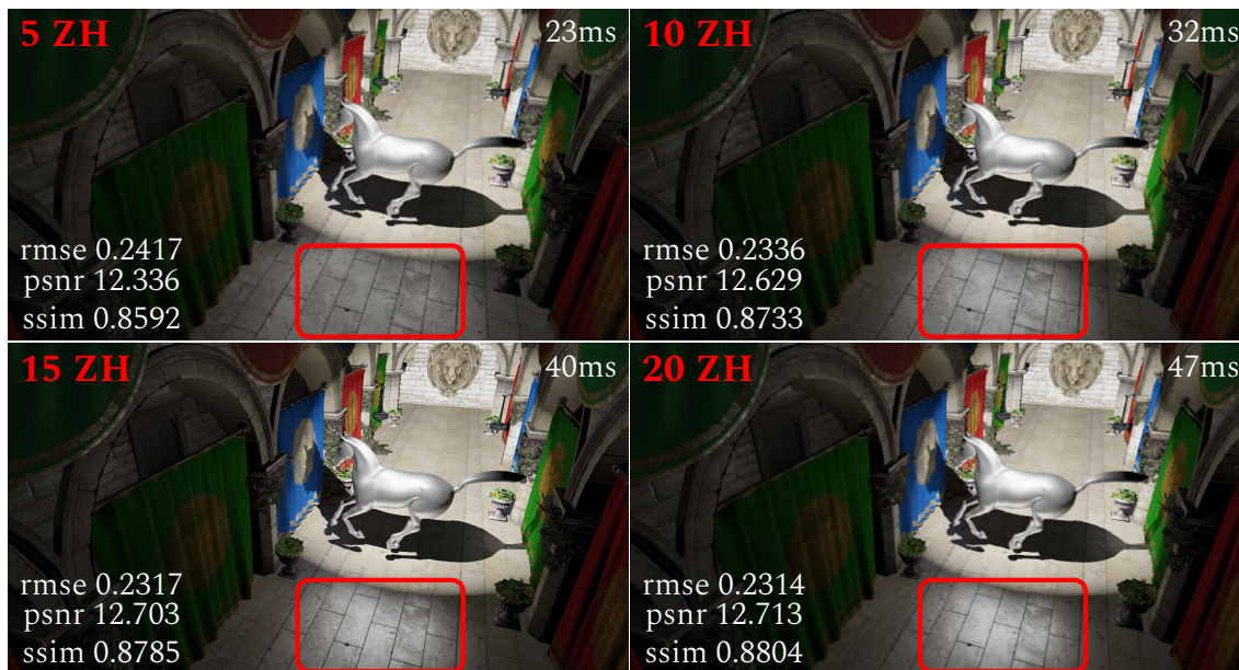
Figure 5.13: Observation of the effect of the number of zonal harmonics using 400 HVLs. We clearly see the specular reflection on the ground becoming higher with higher frequency. However, we can also see that the rendering does not need to go beyond 15 ZH. Indeed, between 15 and 20 ZH, we do not observe any visible difference. The error values show it as well.
