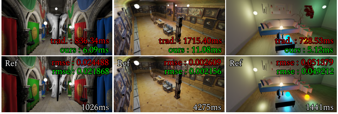
Figure 4.1: Computing per-pixel shading using Spherical Harmonics (SH) is a costly task that requires to compute a SH product when evaluating specular contribution. In this work, we derive a new formulation of this product for decomposable BRDFs. Our approach reduces computation timings by two orders of magnitude and improves the quality of the final image (as measured by RMSE). Top: images obtained with our approach using 9 SH bands. Bottom: Reference images generated by sampling 10,000 rays for each light.
