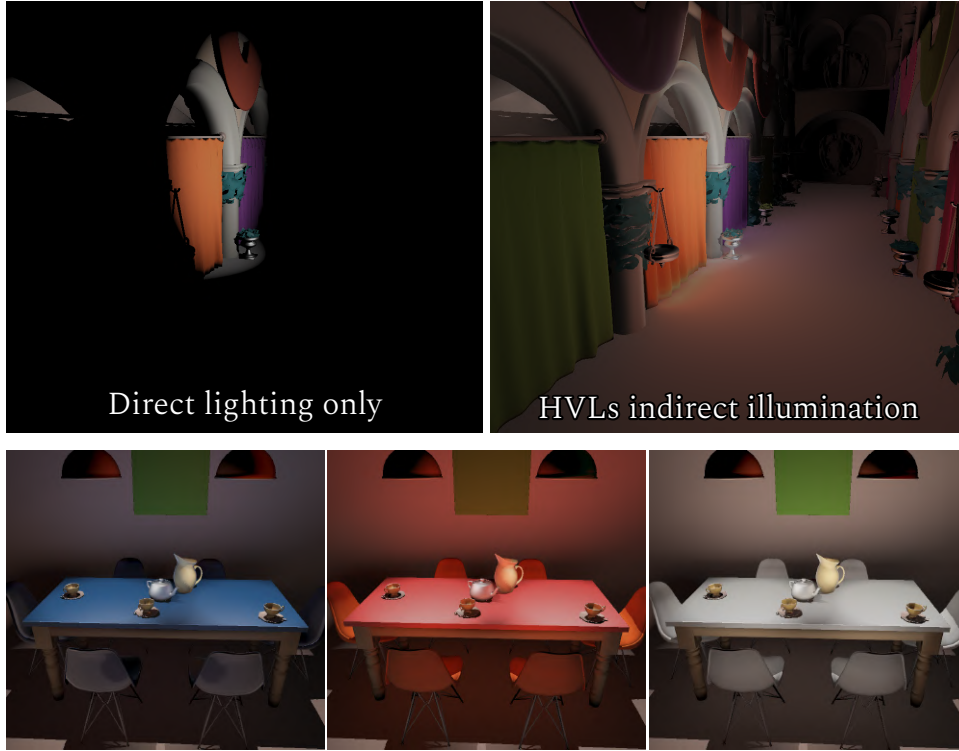
Figure 5.9: Global illumination using HVLs with different measured materials. In our framework, materials can be changed dynamically without affecting rendering time. In the bottom row, only the materials applied to the chairs and the table are modified between the three pictures.
