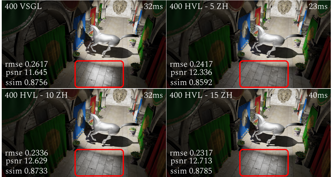
Figure 5.14: Comparison between VSGL and HVL. HVL need use enough ZH bands to match the rendering generated with VSGL.
