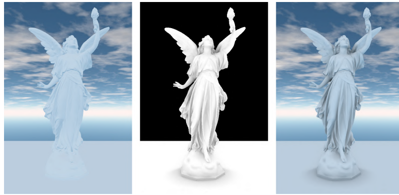
Figure 2.14: The occlusion characterizes the accessibility of a point according to the surrounding geometry (left: without occlusion, middle: only occlusion and right: combination of both). Result given by Jimenez et al. [JWPJ16].
