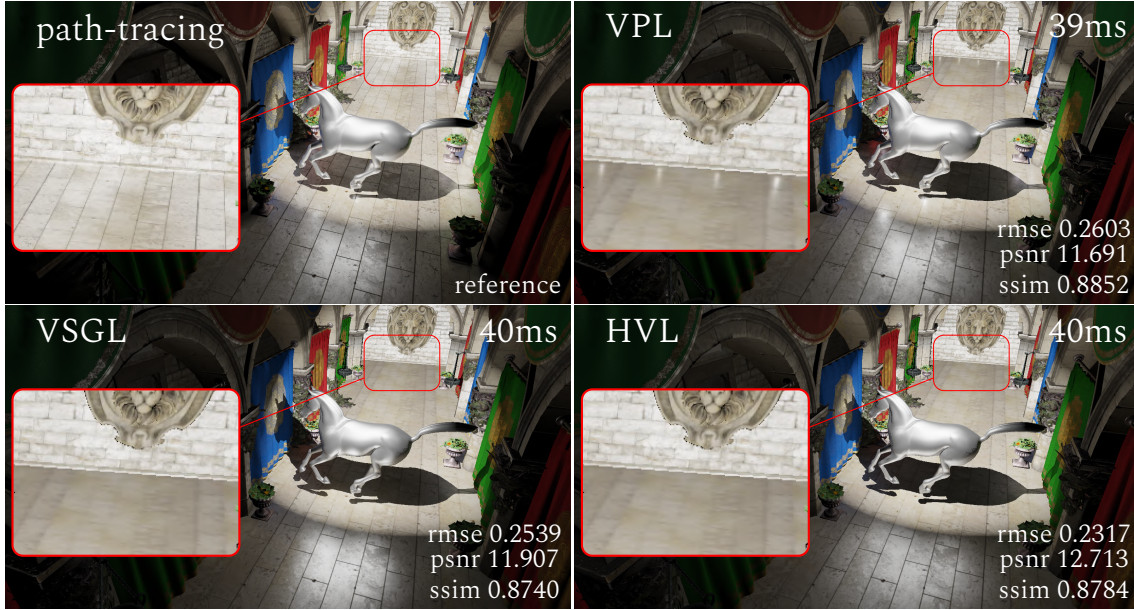
Figure 5.12: Comparison with 900 VPL, 529 VSGL and 400 HVL, generated at equal time. Images are rendered at 1600 \times 900 . The HVL cache resolution is 322^2 pixels, and 14^2 pixels for one VSGL. The contribution of HVLs is on 15 SH bands. In this rendering, HVL are limited to circularly symmetric specular lobe to compute lighting only on ZH. Insets show VPL spike artifacts and VSGL or HVL robustness to those artifacts.
