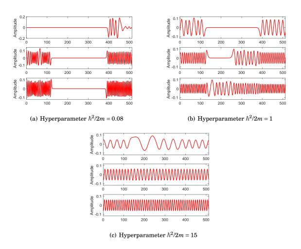
FIGURE 4.8. Role of the hyperparameter  $\hbar^2/2m$ : adaptive basis functions (wave functions) number 25, 70 and 100 calculated from the signal Fig. 4.3 are shown from top to bottom with different values of the hyperparameter  $\hbar^2/2m$ .
