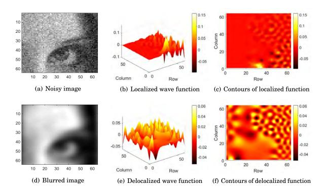
FIGURE 4.6. Role of the hyperparameter  $\sigma$  and localization: (a) *Lena* image used in Fig. 4.1, contaminated by additive Gaussian noise corresponding to a SNR of 15 dB, (b,c) localized wave function number 195 calculated from the noisy *Lena* image (a), (d) blurred version of the noisy *Lena* image in (a) obtained by Gaussian low-pass filter corresponding to  $\sigma^2 = 6$ , (e,f) the same wave function but delocalized due to the low pass Gaussian filter applied to the noisy image.
