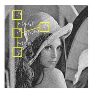
FIGURE 3.7. Principle of Non-Local Means filtering algorithm. Similar pixel neighborhoods give a large weight,  $w(\bar{z}, z_1)$  and  $w(\bar{z}, z_2)$ , while much different neighborhoods give a small weight  $w(\bar{z}, z_3)$ .
