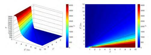
(b) Number of significant wave vectors  ${\mathcal T}$  for different values of the hyperparameters  ${\mathcal E}$  and  $\hbar^2/2m$
