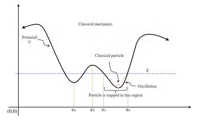
FIGURE 2.1. Motion of a classical particle with an energy E under a potential V. The blue dashed line represents the energy of the classical particle.
