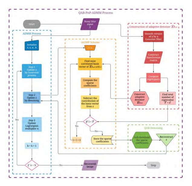
FIGURE 5.2. Flowchart of the proposed QAB-PnP algorithm.
