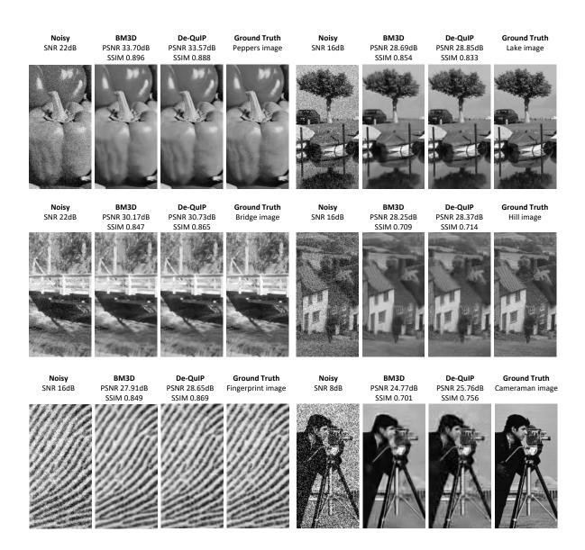
FIGURE 6.9. The Gaussian denoising results for different level of noise. The noisy, BM3D results, De-QuIP results, and ground-truth images are presented here accordingly. The BM3D and De-QuIP schemes are listed as these are always among the two best-performing methods.
