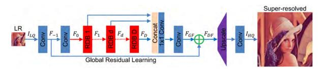
FIGURE 3.10. The architecture of a residual dense network for image superresolution [414].
