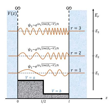
FIGURE 2.6. Wave functions of a particle in a nonzero potential box. Three wave functions and respective energy levels are shown. The frequency of the wave functions are proportional to  $\sqrt{E_r - V}$ , with  $E_r > V$ .
