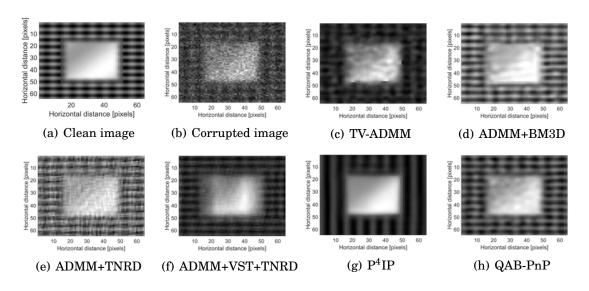
FIGURE 5.10. Deconvolution result for Synthetic image, blurred by a Gaussian kernel  $h_{\sigma=5}^{4\times4}$  and corrupted by Poisson noise corresponding to a SNR of 15 dB. The proposed QAB-PnP algorithm used  $\mathscr{E} = 4.1$ ,  $\lambda_0 = 1.3$ ,  $\hbar^2/2m = 4$  and  $\gamma = 1.01$ ,  $\sigma_{\mathcal{QAB}} = 7$ .
