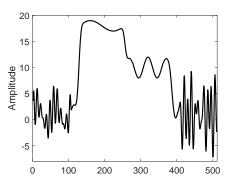
FIGURE 4.3. Synthetic signal used to illustrate the localization property of the wave functions.
