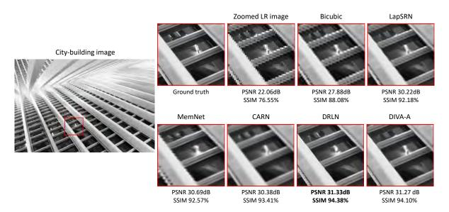
FIGURE 7.15. A zoomed regions of the restored HR *City-building* images, extracted from SR results for a bicubic downsampling with scaling factor 3.
