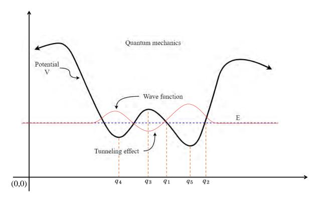
FIGURE 2.9. Wave function with energy E under a smooth potential V. The blue dashed line represents the energy of the quantum particle.
