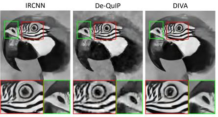
PSNR 24.40dB/SSIM 72.41% PSNR 22.97dB/SSIM 70.34% PSNR 24.87dB/SSIM 85.69%
