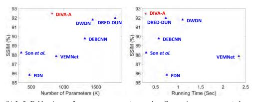
(b) Left: Deblurring performance vs parameter number. Comparisons are presented on the Levin dataset with motion blur and  $\sigma = 7.65$ . Right: Deblurring performance vs run time. Comparisons presented on the Levin dataset with motion blur and  $\sigma = 7.65$ .
