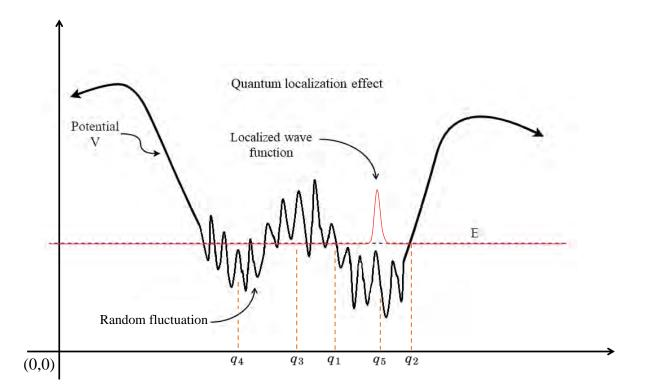
FIGURE 2.10. Slaking wave function with energy E under a random potential V. The blue dashed line represents the energy of the quantum particle.
