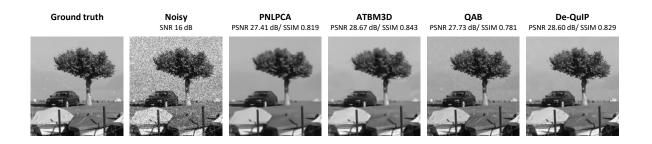
FIGURE 6.12. Zoomed segments of the denoised estimations of the *Lake* image while corrupted with Poisson noise (SNR 16dB) using different methods.
