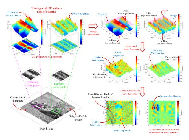
FIGURE 5.1. Relationship between the clean and noisy images under the quantum mechanical framework and their effects on the wave functions: example of the *Boat* image.
