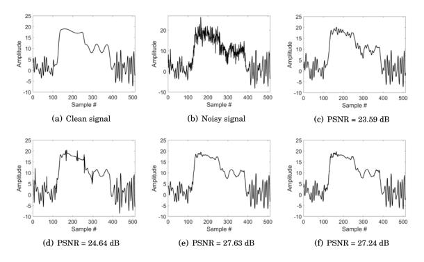
FIGURE 8.1. Denoising results using a quantum algorithm (prototype) for synthetic signal corrupted with Poisson noise corresponding to a SNR of 15 dB.
