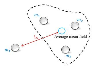
FIGURE 2.12. Interaction between a particle and the average mean-field.
