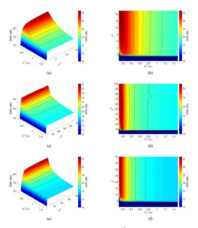
FIGURE 4.11. Influence of the hyperparameters  $\hbar^2/2m$  and  $\sigma$  on the proposed decomposition performed on the 1D system Fig. 4.3 in presence of (a,b) Poisson noise, (c,d) Gaussian noise and (e,f) speckle noise corresponding to a SNR of 15 dB respectively. The hyperparameters are  $\rho = 1$  and s = 110 for each set of experiment.
