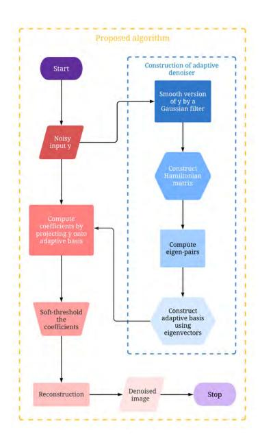
FIGURE 4.7. Flowchart of the proposed denoising algorithm.
