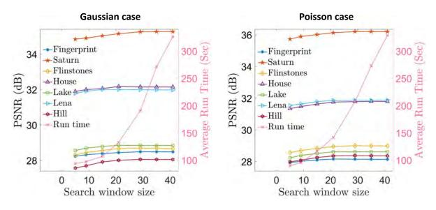
FIGURE 6.4. Denoising performance in terms of PSNR (left y-axis) and average run time (right y-axis) of De-QuIP as a function of the search window size for the first seven sample images in Fig. 6.3. The images hyperparameters  $P_h = 7$  and others are estimated from the equations (6.9)-(6.12).
