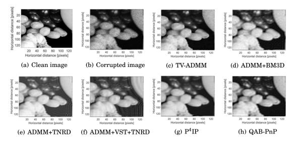
FIGURE 5.11. Deconvolution result for Fruits image, blurred by a Gaussian kernel  $h_{\sigma=3}^{4\times4}$  and corrupted by Poisson noise corresponding to a SNR of 20 dB. The proposed QAB-PnP algorithm used  $\mathscr{E} = 4.5$ ,  $\lambda_0 = 3.15$ ,  $\hbar^2/2m = 4.3$  and  $\gamma = 1.01$ ,  $\sigma_{\mathscr{QAB}} = 8$ .
