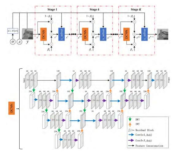
FIGURE 3.11. The architecture of a deep learning-aided inference system for image restoration using the DCNN network as the RED denoiser in the iterative algorithm [194].
