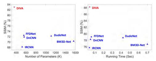
(a) Left: Denoising performance vs parameter number. Comparisons are presented on the BSD68 dataset with  $\sigma = 50$ . Right: Denoising performance vs run time. Comparisons are presented on the Set12 dataset with  $\sigma = 50$ .
