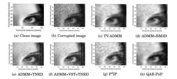
FIGURE 5.9. Deconvolution result for Lena image, blurred by a Gaussian kernel  $h_{\sigma=3}^{4\times4}$  and corrupted by Poisson noise corresponding to a SNR of 10 dB. The proposed QAB-PnP algorithm used  $\mathscr{E} = 3.9$ ,  $\lambda_0 = 1.5$ ,  $\hbar^2/2m = 4$  and  $\gamma = 1.01$ ,  $\sigma_{\mathscr{QAB}} = 7$ .
