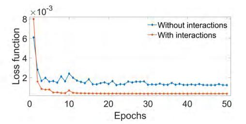
FIGURE 7.3. Loss function (MSE) with respect to epochs. Two specific models are trained for image denoising with  $\sigma = 15$ , with and without integrating the interaction layer in the proposed DIVA architecture for the ablation study.
