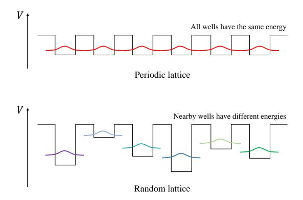
FIGURE 2.8. Periodic and random lattices. Here different colors represent different potential energies.
