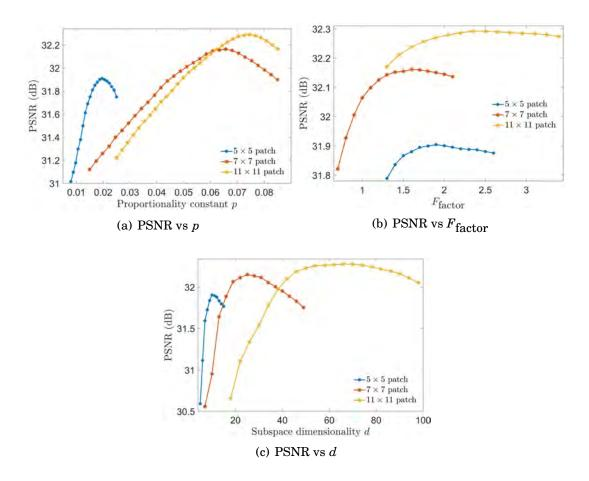
FIGURE 6.5. Denoising performance of De-QuIP in terms of PSNR as a function of the hyperparameters for the *House* image corrupted with AWGN (SNR = 16dB) using three different patch sizes. All hyperparameters are estimated using equations (6.9)-(6.12).
