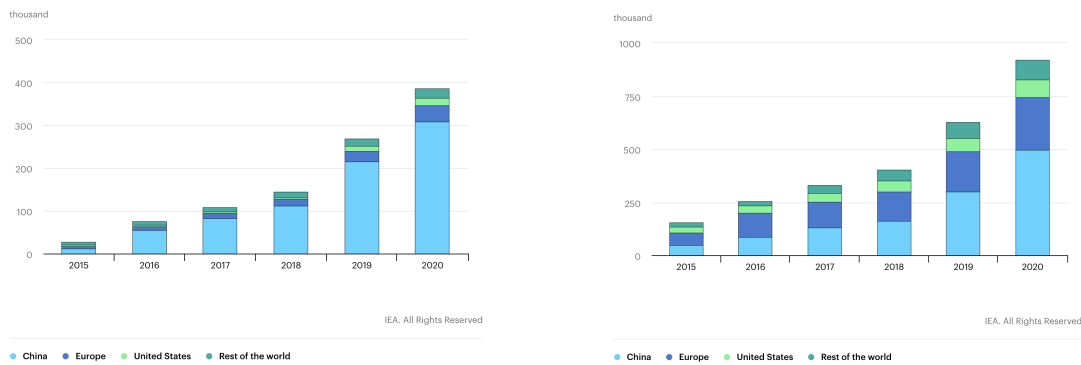
Figure 1.2: Stock of >22 kW (left graph) and <22 kW (right graph) public electric light duty vehicles chargers, 2015-2020 (IEA, 2021a)
