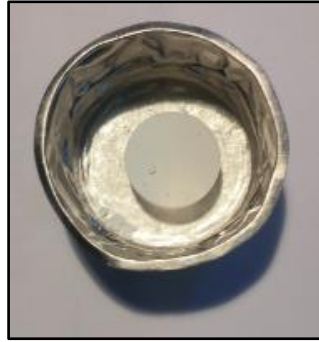
Fig. 26 : Sample in a platinum crucible for heat treatment. For \text{Ca}_2\text{SiO}_4 , heat treatment in pellet form is not required as the pellets change to powder at low temperatures. Nevertheless, the specific reaction area is greater and heat transfer is more homogeneous.
