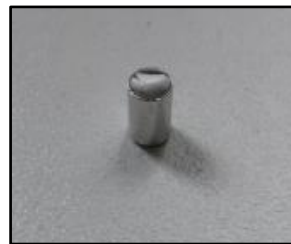
Fig. 29 : \text{Ca}_2\text{SiO}_4 dusting after DSC measurement.
