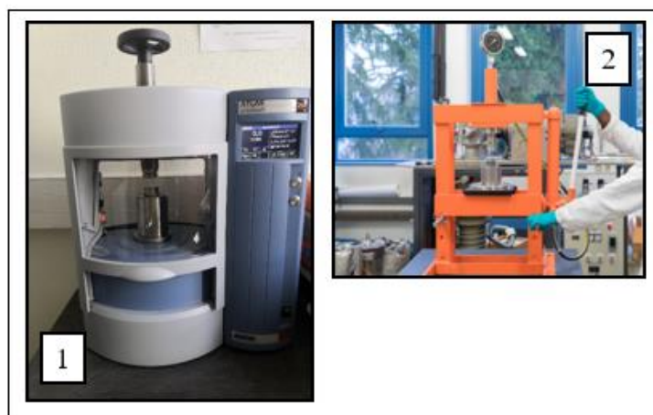
Fig. 1 : Automatic hydraulic work press on the left (1). Manual press on the right (2).
