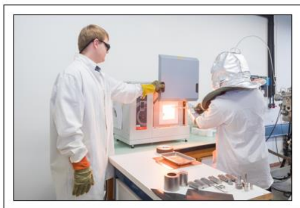
Fig. 2: Silicate synthesis in a platinum crucible under air.
