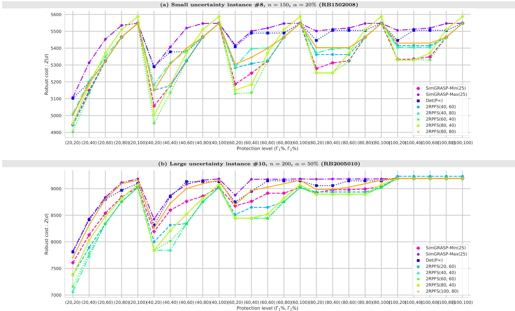
Figure 3.3 – Robust cost of deterministic, 2RPFS and SimGRASP solutions versus protection level ( \Gamma_1\% , \Gamma_2\% ). All presented 2RPFS solutions are optimal.
