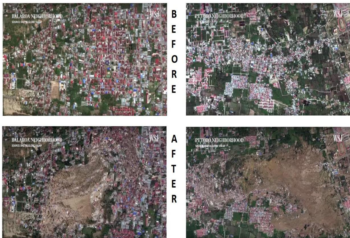
*Figure 1.5 Damage caused by liquefaction at Palu (Sulawesi) – From Reuters Images*
