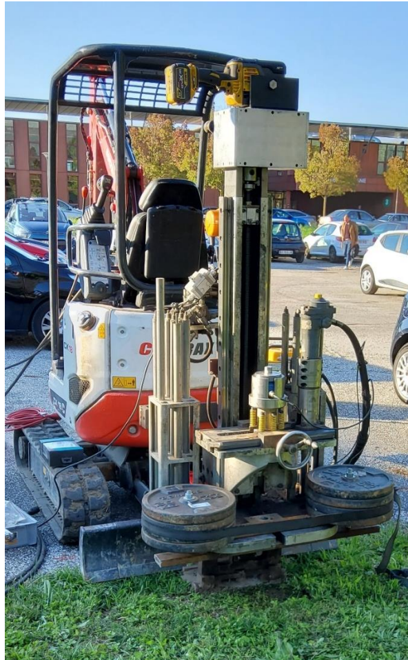
Figure 6.3 Equaterre's new CPT rig
