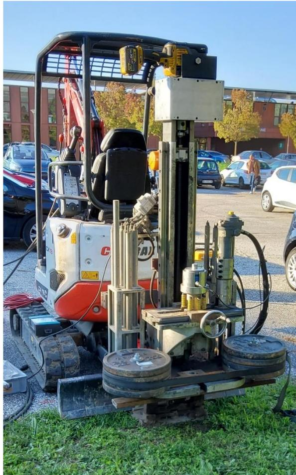
*Figure 6.3 Equaterre's new CPT rig*
