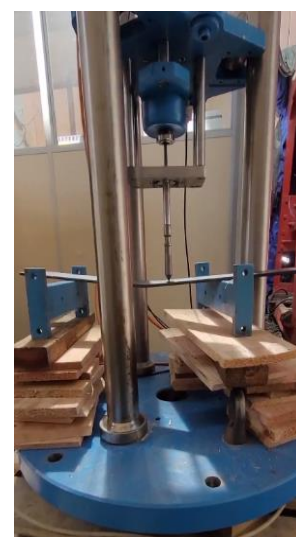
Figure 2.14 Cyclic CPT test being performed on a steel beam
