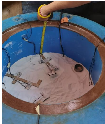
Figure 2.10 Sensor group placement in sand ensuring required radial and vertical positions of sensors.
