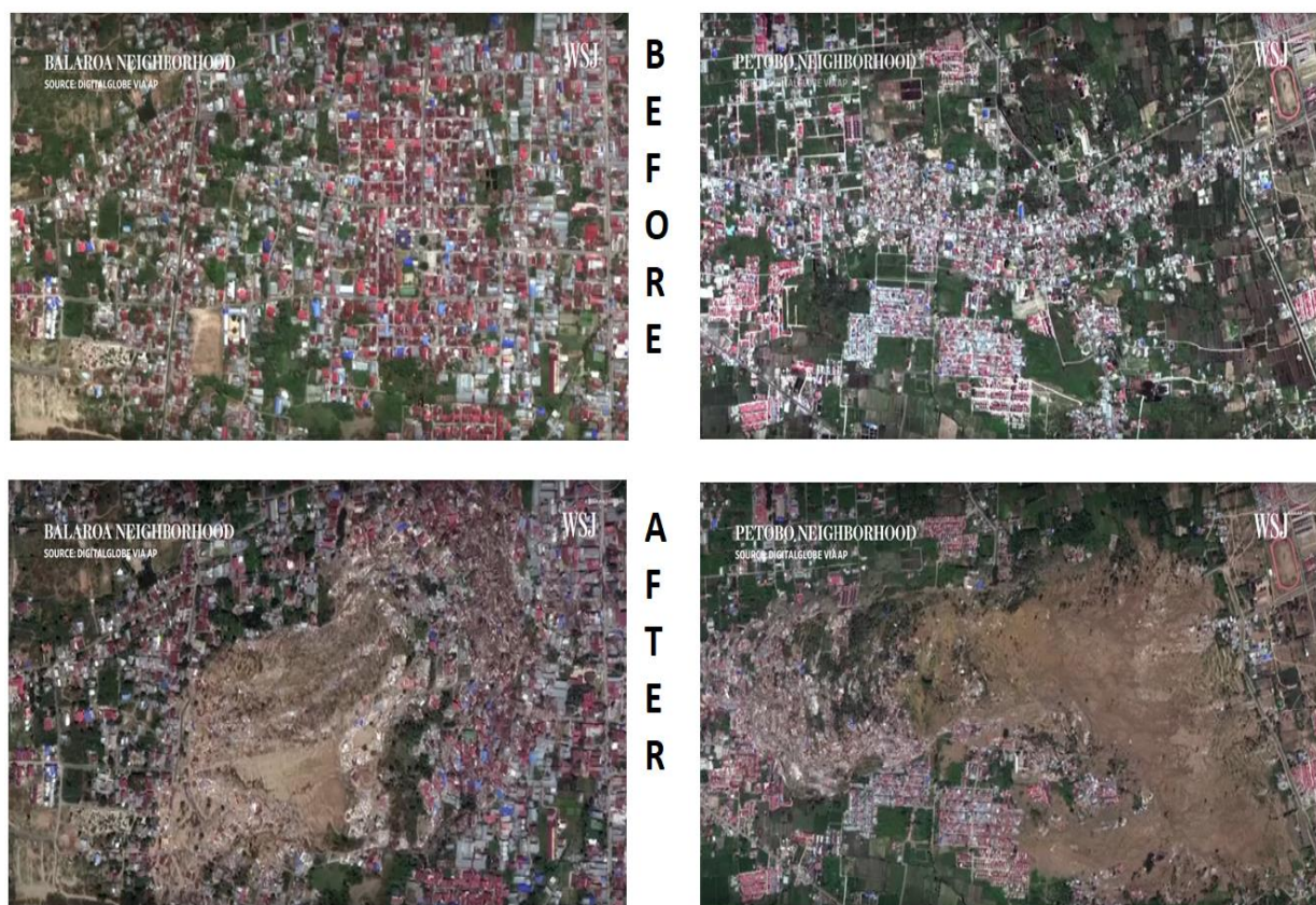
Figure 1.5 Damage caused by liquefaction at Palu (Sulawesi) – From Reuters Images
