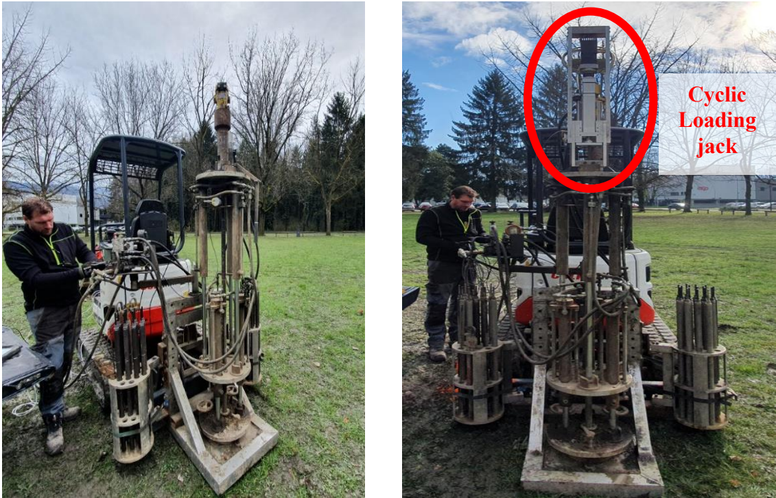
Figure 4.11 CPT pushing rig - Setup for normal driving (left) and for cyclic CPT test (right)
