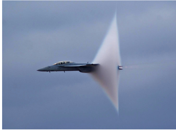
Figure 1.2: Example of a shock wave formed for a jet moving at supersonic speed.
