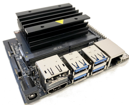
Figure 2.3: Nvidia Jetson Nano 2 Development Kit [21].
