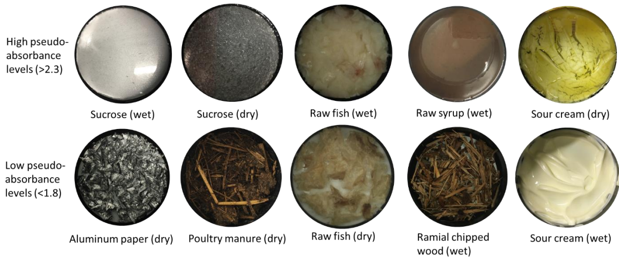
Figure 15. Visual aspect of substrates with low and high levels of pseudo-absorbance. Pictures were taken from above the NIRS measurement cell.
