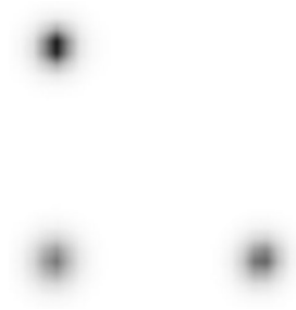
Figure 2. Axial reconstructed slice of the three line sources for the evaluation of the spatial resolution.
