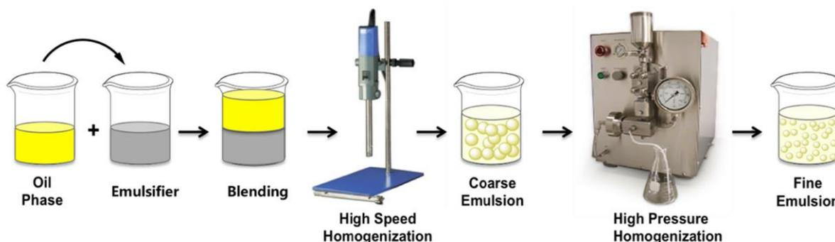
FIGURE 1 The flow chart of the preparation of nanoemulsions
