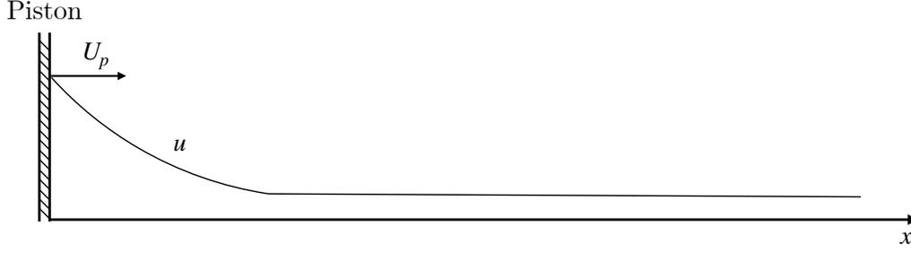
Figure 3.4: Sketch of a one-dimensional inert, inviscid flow pushed by a moving piston.
