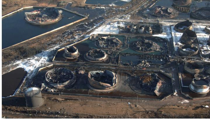
Figure 1.1: Aftermath of the Buncefield fire that took place at a fuel storage facility in the UK in 2005. According to the final investigative report [13], the fire was started by a detonation of a gaseous fuel-air mixture in one of the tanks.
