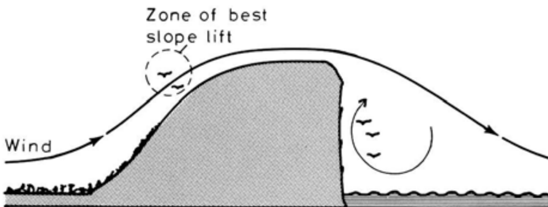
Figure 15: Slope soaring (Pennycuick, 1975). The best lift is found over a smooth slope (left), while vertical cliffs can produce more complicated flow patterns but sometimes give useable lift when facing downwind (right).
