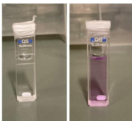
Figure 2.2: Solution of C5HT-di-PSAc at 1.25 \times 10^{-5} \text{ M} in DMF before any irradiation so with most of the molecules are in the open state (colorless solution on the left) and after UV irradiation with most of the molecules in the closed state (purple solution on the right).
