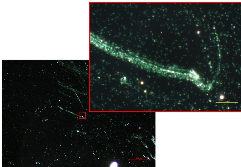
Figure 2.18: Dark field microscopy images with 10x magnification and 100x magnification of single 51 nm AuNPs (the green dots) on ITO (zone B of sample ADITO81). Luminosity 75 %, gain 6.2 x, exposure time 700 ms.
