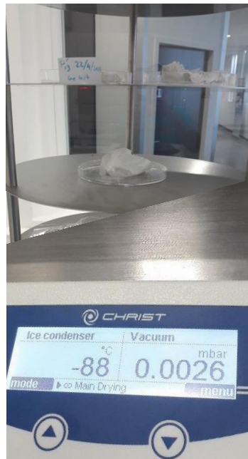
Supplementary figure 1: Fabrication process of the freeze-dried gelatin samples
