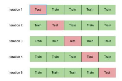
Figure 2.6: 5-fold cross validation example
