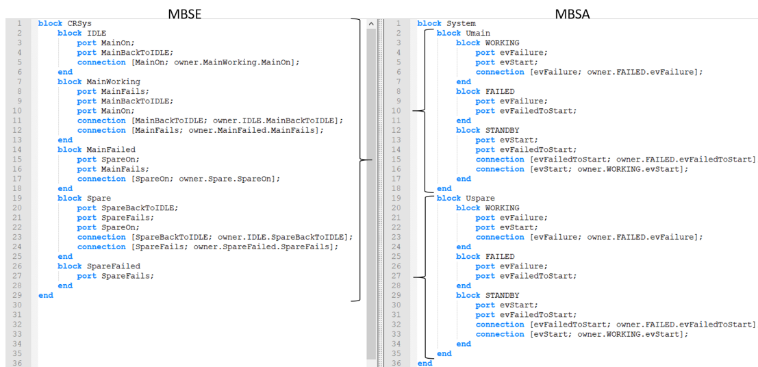
Figure 3.7: S2ML abstractions for the cold redundancy with primary mapping
