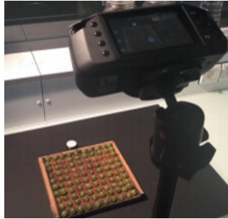
Figure 2. Hyperspectral acquisition of grape berries.
