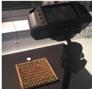
Figure 2. Hyperspectral acquisition of grape berries.
