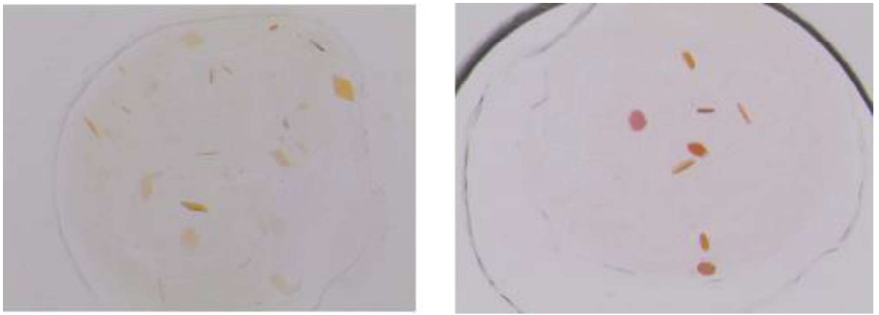
Figure 3.1.4.1 Diamond- (left) and hexagonal- (right) shaped crystals obtained during the crystallisation trials for NpSRII/NpHtrII solubilized in DDM.
