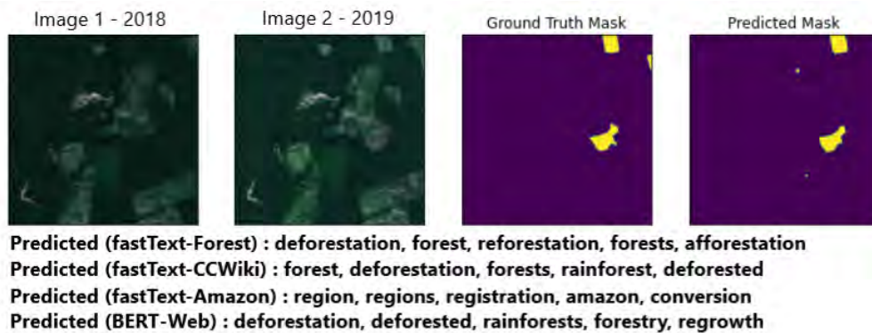
Figure 5.13: An image pair with its ground truth mask and the mask predicted by the change detection model (Section 5.3.2) along with the top five annotations predicted by three visual semantic models. fastText-Forest and BERT-Web correctly predicted the true annotation "deforestation" as the top 1 annotation. fastText-CCWiki produced the correct annotation in second position. These three models predicted forest related words. The fastText-Amazon model does not predict the correct annotation in the top 5 but it predicts the relevant annotation "amazon" in fourth position.
