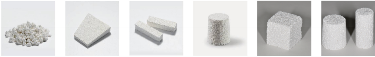
FIGURE 1.5 – Synthetic materials made from hydroxyapatite and tricalcium phosphate produced by the company Biomatlante and used as bone grafts. They are composed of macro- and micropores, with a porosity of 70%, which allows cell and nutrients transport. From biomatlante.com
