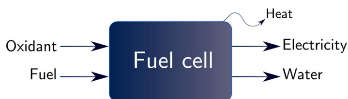
Figure 1.1. Fuel cells' basic operating principle.
