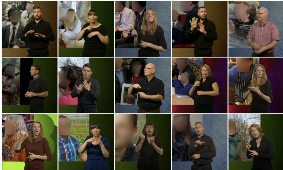
Figure 4.7: Background face blurring. Faces appearing behind the interpreter are automatically tracked and blurred for anonymisation purposes.
